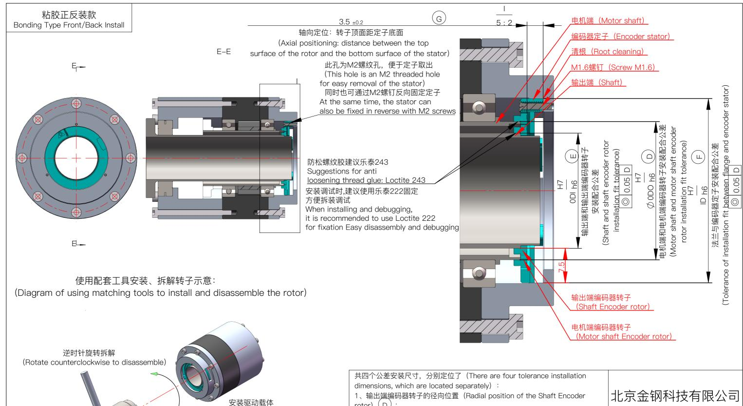
(Installing the driver carrier)
